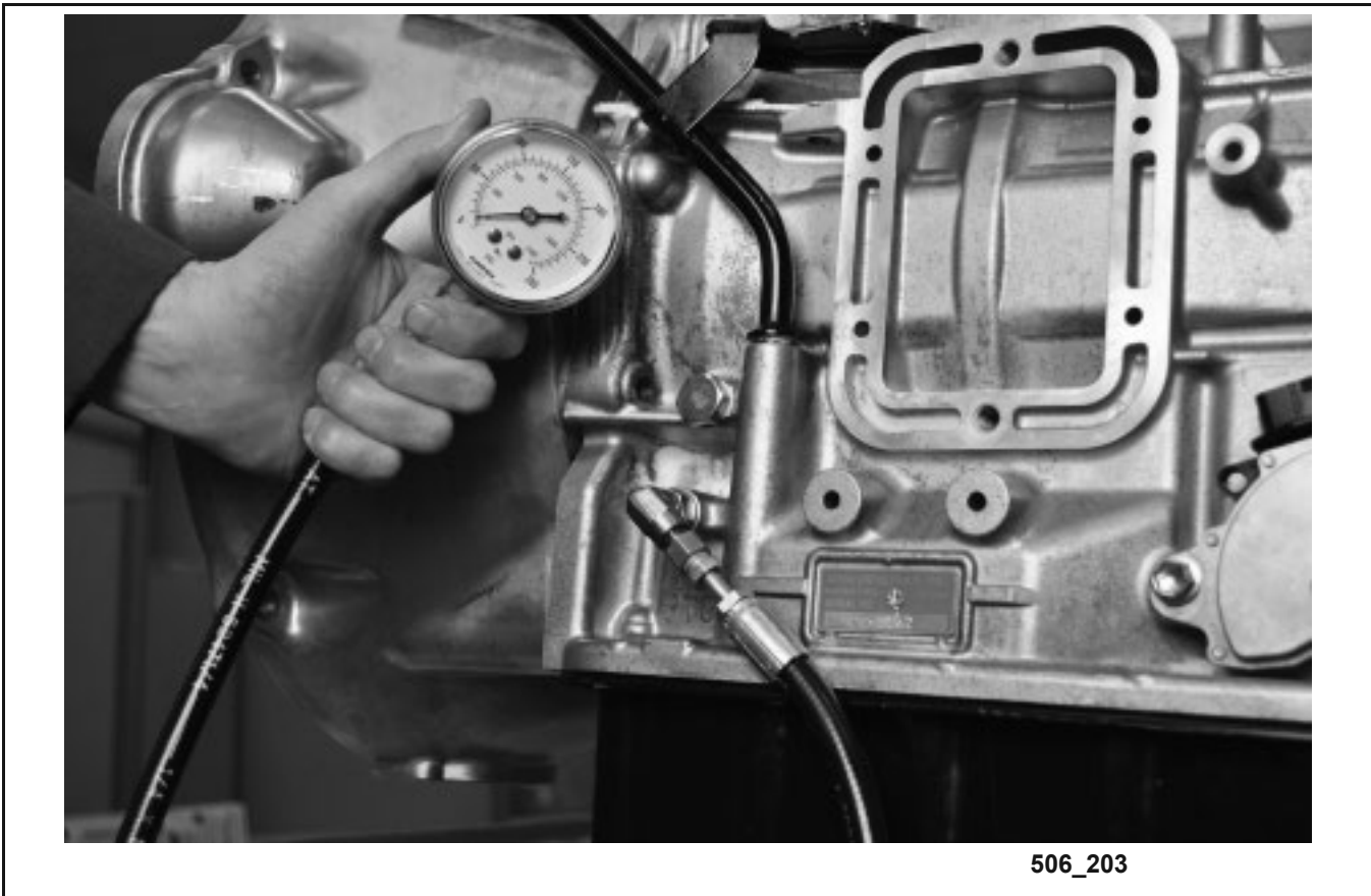
Figure 53 Fluid Pressure Gauge and Line Adapter Attached to Transmission Test Port
