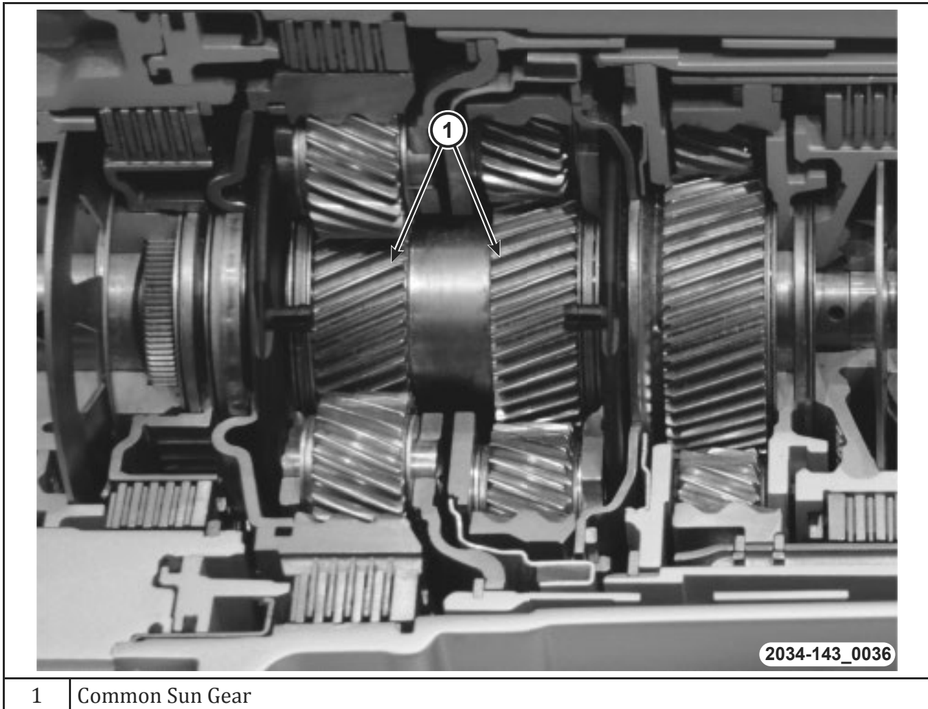
Figure 67 Simpson Gearset (8HP45 P1/P2 shown)
