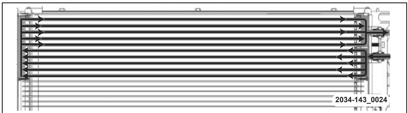
Figure 40 Double-pass Parallel-path Cooler Construction
